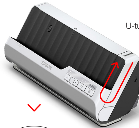
Sliding the position selector button across adjusts the scanner's angle
